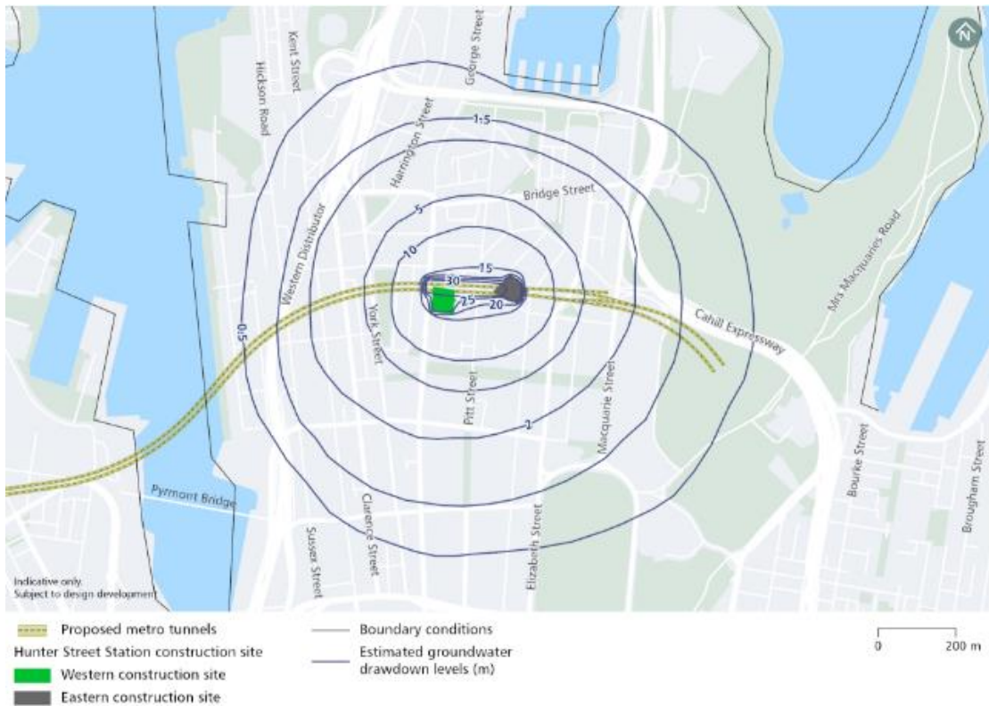
Figure 2-4: Predicted Groundwater Drawdown Levels Two Years After the Start of Construction of Hunter Street Station (SSI EIS 2)
